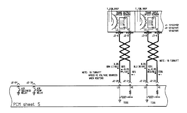
Figure 3.2.1a - III - P/Truck - Mechanization Diagram-VSS (TISS & TOSS), Air Pump & Solenoid Relay
